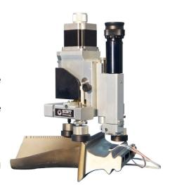
The heart of the system is the alignment-drilling unit, which is used to physically drill the hole and align the cutter with the centre of the strain gage rosette by means of a cross reticule in the eyepiece. The system is also used, at the end of testing, to obtain the measurement of the hole diameter.
